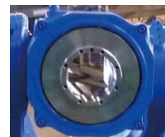
T-axis hollow arm: 50 mm dia.
