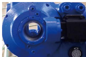
R-axis hollow arm: 50 mm dia.
