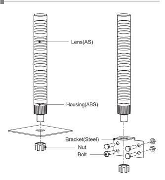
• Machine holes on the mounting surface referring to the diagram below.
