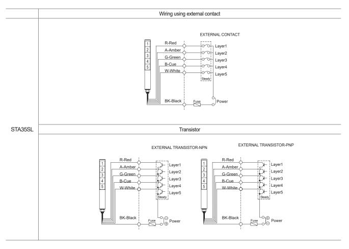
• External power line/ external signal line - UL1007 AWG22(0.3sq) 400mm
