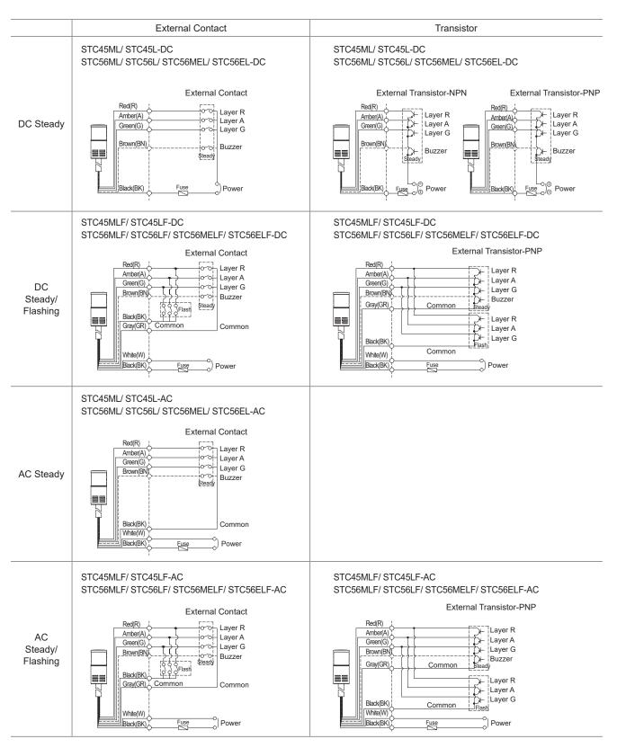
• DC steady type cable specification : External power/ signal line - UL1007 AWG22(0.3sq) 400mm
