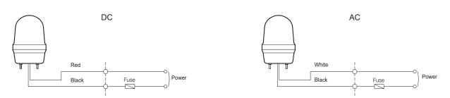
• External power line - UL1015 AWG18(0.75sq) x 2C 400mm.
