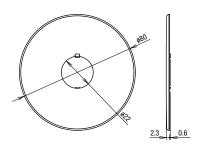
• Panel thickness when using the nameplate: 0.8 to 4 mm
